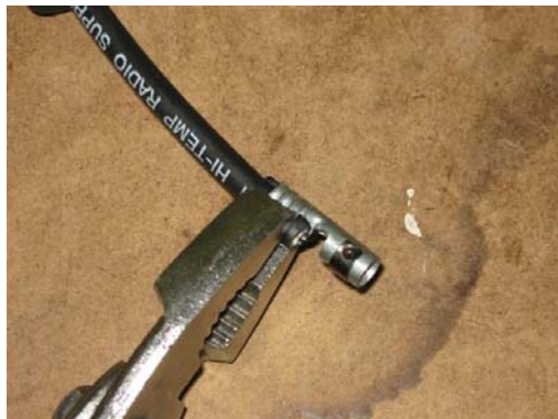
11. Position terminal on wire. Squeeze terminal sides with pliers.
