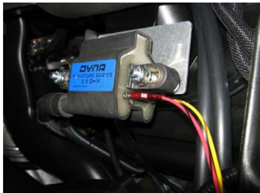
21. Mount Dyna coil. Attach plug wires and primary wires. Red to red dot. Yellow to no dot.
