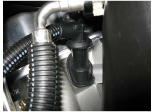
16. Slide boot over #1 spark plug.
