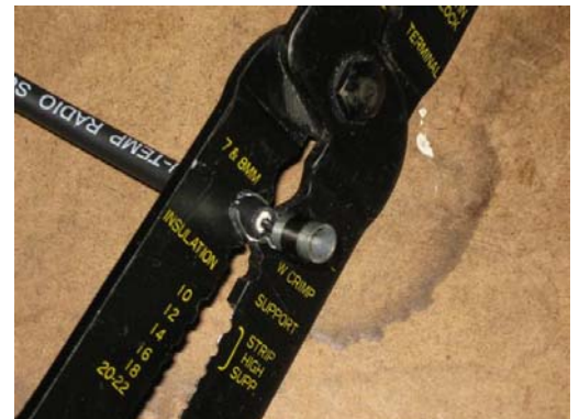
12. Position crimp tool on terminal. Squeeze terminal until crimp is secure.
