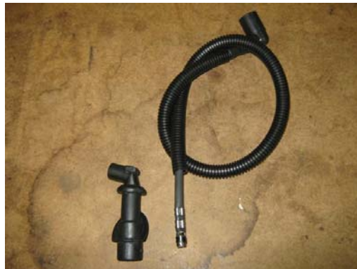
3. Original Boot, pulled off.
