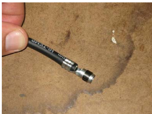
13. Terminal after crimping.
