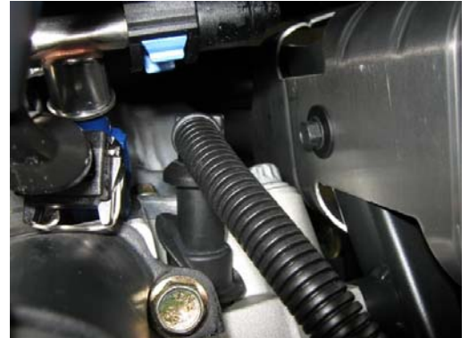
18. Slide boot over #2 spark plug.
