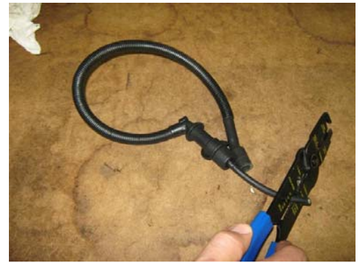
8. Strip insulation off carbon core.
