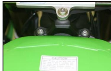
5. Remove fuel tank by supporting tank in the up right position and disconnecting the fuel line and fuel pump connector. Also remove all vent hoses.
