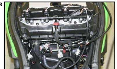
10. Ground the JUICE BOX™ wire to the battery (-) terminal. (Fig. 9)
