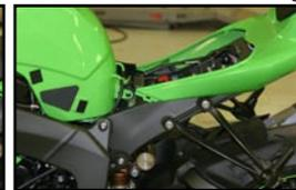
4. Remove both fuel tank bolts from front of fuel tank and rotate steering damper out of the way. (Fig. 5)
