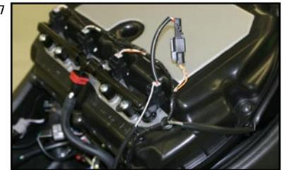
9. Locate the 4 lower injectors and unplug the grey connectors. Plug the JUICE BOX™ grey connector into the injector and its pig tail into the OEM wire for that connector. (Fig. 8)
