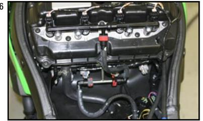
8. Disconnect one upper injector and plug the black connector from the JUICE BOX™ into here. Plug the OEM harness into the pig tail male end of this wire. (Fig. 7)
