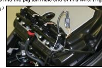
Locate the 4 lower injectors and unplug the grey connectors. Plug the JUICE BOX™ grey connector into the injector and its pig tail into the OEM wire for that connector. (Fig. 8)
