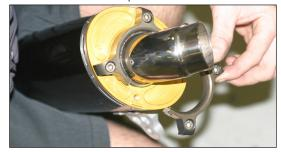
6. Install left muffler using the OEM hardware and springs.
