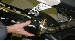
7. Install right muffler using the OEM hardware and springs.
