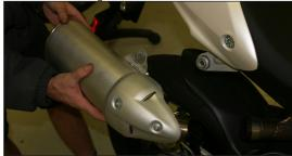
Install TBR slip-on tubes to mufflers by attaching the X-Ring to the mufflers using the 6x14mm socket head cap screws and lock washers provided. Leave loose for now.
