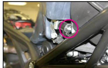
7. Remove bottom tank bolt. (fig.5)
