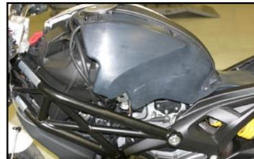
6. Remove fuel tank by removing lower bolt that secures tank from sliding rear-ward. (fig.4)
