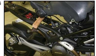
9. Locate left injector and unplug OEM connector and plug in the JUICE BOX™ female end into the injector and male end into the OEM harness. (fig.7)
