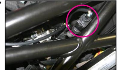
10. Locate right side injector and pass wire through engine compartment to plug into the left side injector and the male end into the OEM harness. (fig.8)
