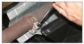
7. Remove muffler assembly.
