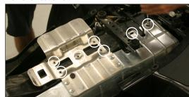
6. Loosen muffler joint clamp.
