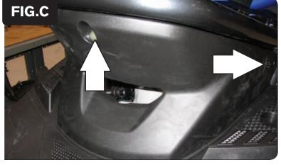
Remove the engine cover by removing the 1 screw in the front and the 2 push tabs (1 on either side) (Fig.C).
