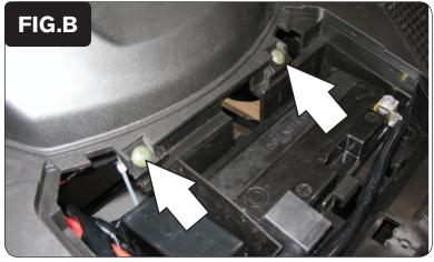
2 Remove the 2 screws shown in Figure B.
