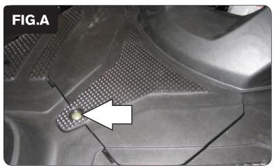
1 Remove the battery cover (Fig. A).
