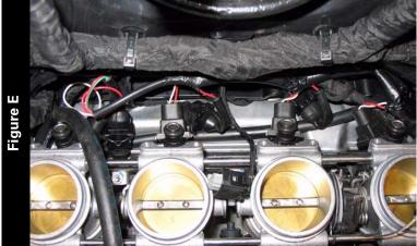
Lay the Juice Box Pro in the tail section and route the harness down the right hand side of the bike towards the throttle bodies.
