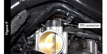
6 Locate the stock throttle position sensor (TPS) connector.
