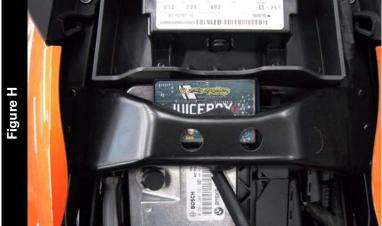
12 Using the supplied velcro, secure the Juice Box Pro in the tail section as shown in Figure H.
