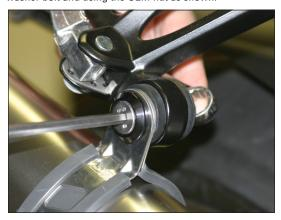
Check alignment of muffler and tighten the 4 6x20mm socket head cap screws on each side. Then tighten barrel clamps and lastly tighten muffler mounts.
