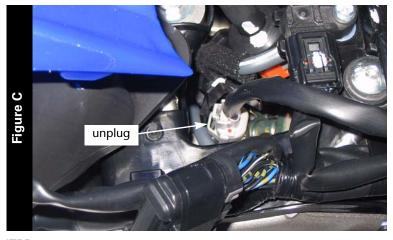
7 Unplug the stock wiring harness from the injector as shown in Figure C.
