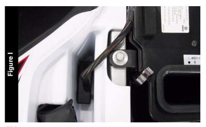
13 Using the supplied velcro, secure the Juice Box Pro in the pocket of the rear fender on the left side as shown in Figure I.
