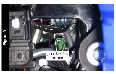
Route the 3-pin connectors from the Juice Box Pro harness down the left side of the throttle body as shown in Figure D.
