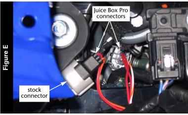
Attach the Juice Box Pro wiring harness to the fuel injector and the stock wiring harness as shown in Figure E.
