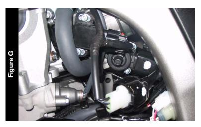
11 Attach the Juice Box Pro wiring harness to the stock TPS and wiring harness as shown in Figure G.
