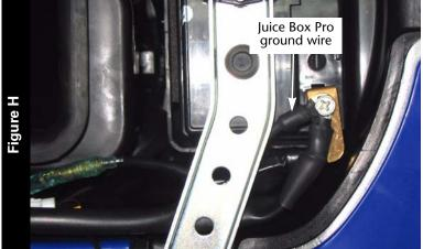
12 Attach the ground wire from the Juice Box Pro to the negative side of the battery as shown in Figure H.
