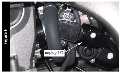
10 Unplug the throttle position sensor (TPS) connector from the left hand side of the throttle body as shown in Figure F.
