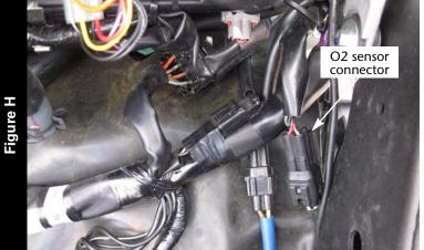
13 Locate the stock O2 sensor connector.
