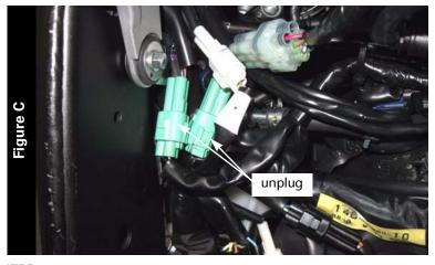
7 Unplug the 3-pin and 4-pin green connectors from the throttle bodies to the main wiring harness as shown in Figure C.
