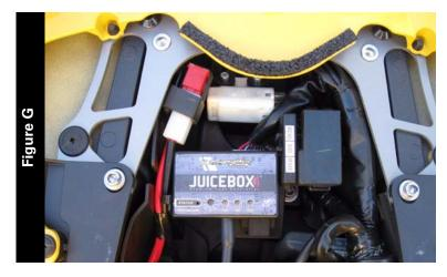
12 Using the supplied velcro, secure the Juice Box Pro in the tail section of the bike as shown in Figure G.
