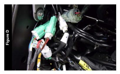
Attach the Juice Box Pro connectors to the throttle bodies and stock wiring harness as shown in Figure D.
