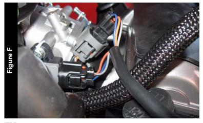
12 Attach the Juice Box Pro connectors to the TPS connector and stock wiring harness as shown in Figure F.
