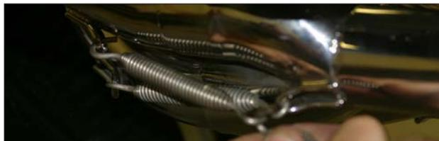
13. Install supplied muffler mounting bracket to previously installed longer bolt behind right side foot rest. The bracket goes on the inside and is held in place with the supplied nut.
