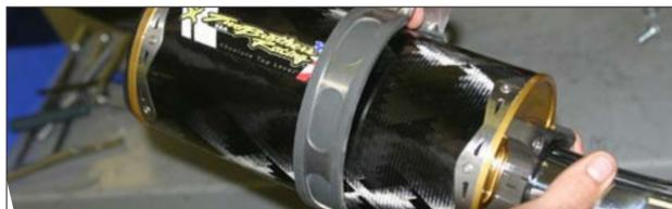
16. Locate the muffler mounting bracket previously installed and rotate slip-tube and muffler to desired location, secure to muffler mounting bracket (There is a lot of adjustment because the bracket / clamp / muffler and slip-tube may all be moved individually so keep in mind the muffler should be as close to the swingarm as possible without touching leaving a minimum of 1/4" clearance).
