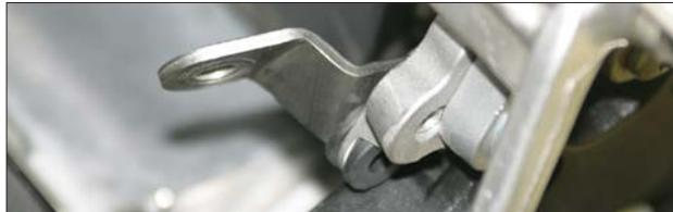
14. Attach TBR muffler to supplied slip-on tube using the 2 part X-ring and 6x14mm socket head cap screws and lock washers provided, leave loose for now.
