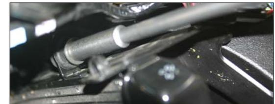
6. Remove servo cables and pulley wheel from servo motor on left side of motorcycle. **You must use a suitable tool to hold pulley wheel in place while removing retaining bolt.**
