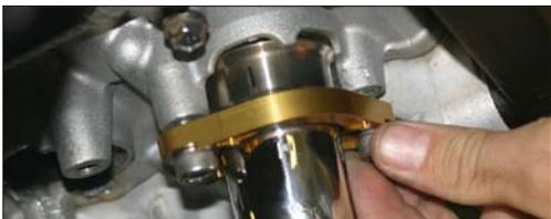
11. Install collector assembly. Use gasket maker on all slip-fit joints.
