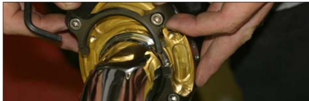
15. Install rubber lined muffler clamp over TBR muffler and slide muffler assembly over TBR header making sure the supplied barrel clamp is on the slip-tube where the exhaust joint will be.
