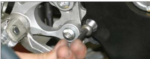
10. Install TBR header 1-4, 1 being the left and 4 being the right if sitting on the bike. Keep loose for now (make sure to use the OEM copper gasket between cylinder head and exhaust header).
