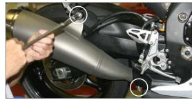
3. Remove OEM plenum box and O2 Sensor.
