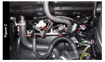
Attach the Juice Box Pro connectors to each injector and the stock wiring harness as shown in Figure C.
