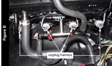
5 Unplug the stock wiring harness from each of the lower injectors as shown in Figure B.
