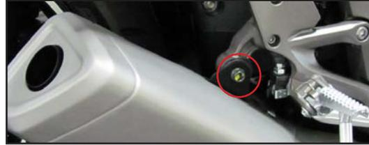
3. Remove the OEM rubber grommet and sleeve from OEM muffler mounting location. This will not be reused.
