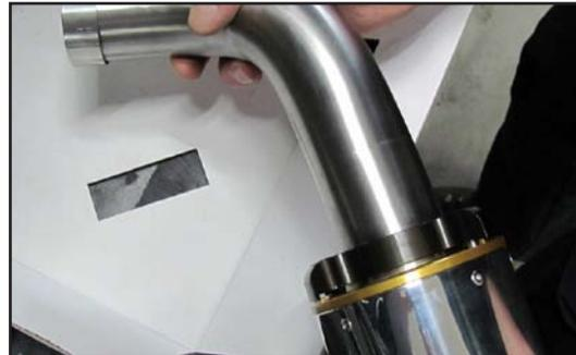
8. Install on motorcycle and attach using the OEM muffler mounting bolt.
