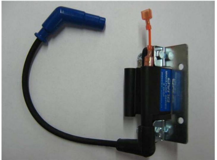
Step 1: Assemble Dyna coil with bracket and wires.
