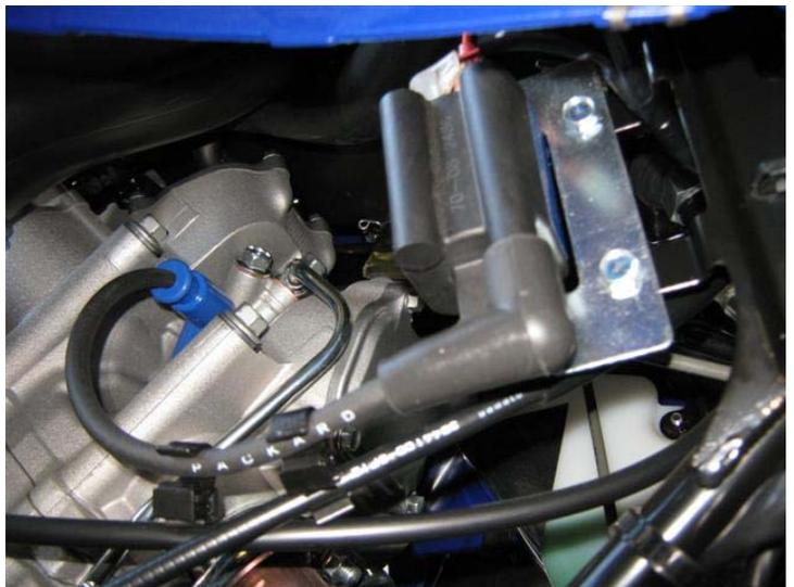
Step 2: Mount Dyna coil assembly to frame.
