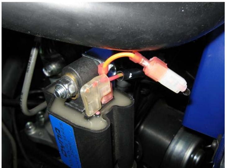
Step 3: Attach coil primary wires.
