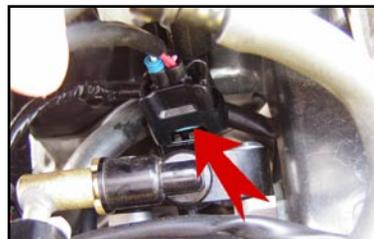
6. Plug the JUICE BOX™'s black male connector into the original white connector you removed in step 3. (Fig 4)
