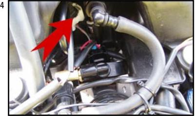
7. Now find a good chassis ground to attach the Juice Box's ground lead. **NOTE: Gas tank mounting bolt or the negative side of the battery.**
