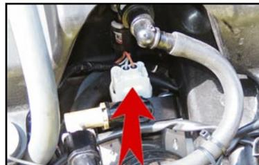
5. Plug the Juice Box's black female connector onto the injector. (Fig 3)
