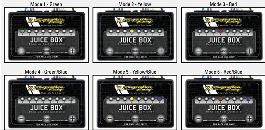
**Additional Tested Setting:** LTR-450 with stock airbox, TBR Slip-on exhaust with spark arrestor and JUICE BOOST™. (G=0.5, Y=1, R=1, GB=8, YB=4, RB=4)
