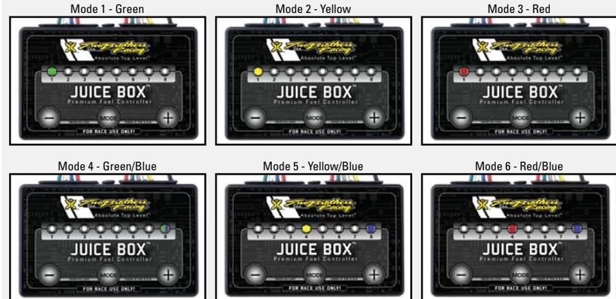
**Additional Tested Setting:** LTR-450 with stock airbox, TBR Full System exhaust with NO spark arrestor. (G=1, Y=4, R=4, GB=8, YB=4, RB=4)
