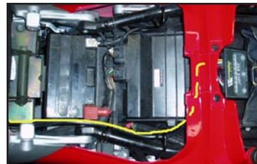
5. Locate the LOWER injector connectors. One at a time, unplug the LOWER injector connectors and plug in the JUICE BOX™ female and male connectors into the injectors and OEM injector connectors that were just disconnected. DO NOT connect the JUICE BOX™ to the upper injectors. (Fig 3)
