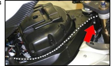
6. Disconnect the LOWER injector connectors from the LOWER injectors. Connect the JUICE BOX™ female and male connectors to the injectors and the injector connectors that were just disconnected. Do NOT connect the JUICE BOX™ to the upper injector connectors. Route the JUICE BOX™ ground lead (black wire) to the exhaust butterfly valve servo bracket that connects to the inside of the right frame spar and connect. (Fig 5)
