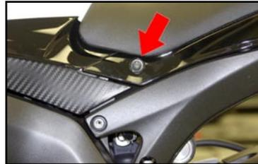
3. Remove the six plastic pop rivets that secure the rear seat fairings and remove the rear seat fairings. The rear turn signals are integrated into the seat fairings so the turn signal wire connectors will need to be disconnected to remove the fairings. (Fig 2)
