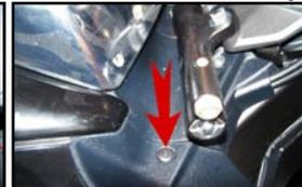
6. Twist and remove ignition cover from ignition cover and remove 5 Allen bolts (Fig 6). Lift housing to gain access to the two connectors and disconnect.
