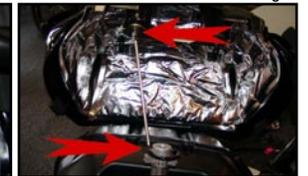
9. Locate lower injectors. *Note: This bike is equipped with two sets of injectors lower and uppers we are only concerned with the lower injectors* (Fig 10). Disconnect injector connector and plug the black JUICE BOX™ connector onto the injector and plug the black connector from the JUICE BOX™ into the stock black connector. Repeat on remaining 3 cylinders.
