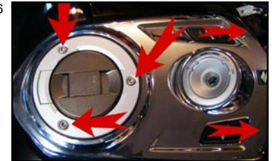
7. Remove (4) Allen screws remove covers and (2) 8mm socket head tank bolts (Fig 7).
