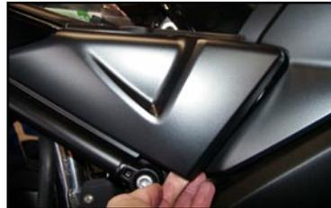
4. Remove screw from tank panel, both sides (Fig 2).
