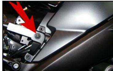
5. Remove Allen screw from front turn signal housing (Fig 3) and two plastic fasteners (Fig 4-5), and remove housing. Repeat on opposite side.
