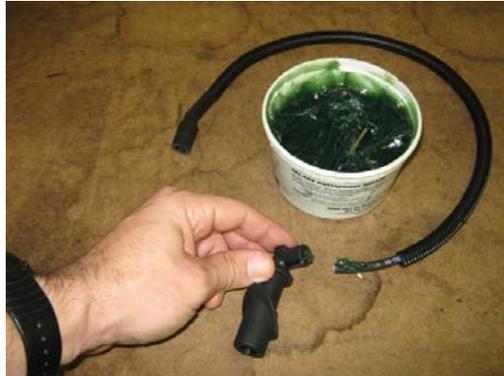
3. Grease wire and spark plug cap.
