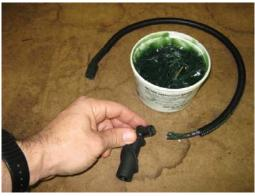
3. Grease wire and spark plug cap.
