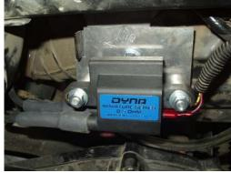
6. Install Dyna coil. Attach spark plug wires.
