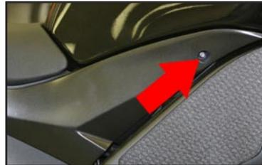
3. Remove the front seat by removing the left and right seat bolts. (Fig 2)
