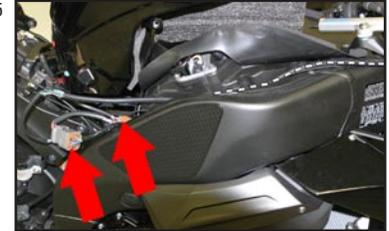
7. Pull the brown 16 pin block connector up from behind the air box, disconnect and connect the JUICE BOX™ connectors to this connector. Route and attach the ground lead (black wire) to the frame ground under the tank at the back of the air box. (Fig 6)
