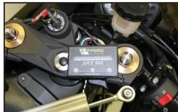
6. Gently rotate the tank back and support. Route the JUICE BOX™ harness between the right fork tube and the steering stem, over the frame and into the engine compartment. The harness can be tucked in between the air box and the frame. (Fig 5)
