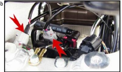
6. Remove the bolt that secures the stock ground wire to the frame. Attach the ground wire from the Juice Box to this location. (See Fig. 5)
