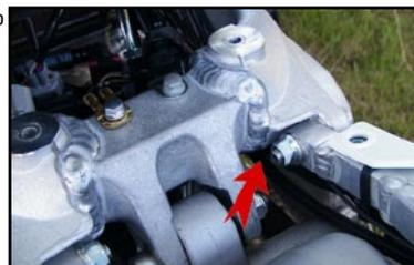
5. Unplug the stock injector connector from the injector. (See Fig.4a) The stock injector connector looks just like the gray connector on the Juice Box. This connection is under the rear of the fuel tank. Plug the Juice Box gray injector connector into the injector, then plug the stock injector connector into the black Juice Box connector. (See Fig. 4b)
