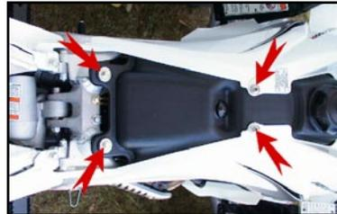
4. A Good location for the Juice Box is in the tail section. Route the wiring harness from the Juice Box towards the throttle body. (See Fig.3a) Route the harness underneath the cross member of the sub frame. (See Fig.3b)
