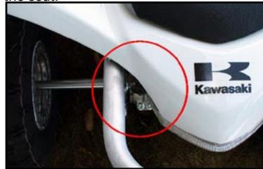
3. Remove the 2 screws that hold the side covers to fuel tank. Remove the 2 bolts at the rear of the fuel tank. This allows the rear of the fuel tank to be raised up enough to install the Juice Box without removing the fuel tank. (See Fig.2)
