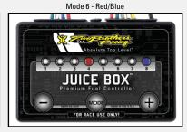
Additional Tested Setting: KFX450R with stock airbox, TBR Slip-on exhaust with NO spark arrestor and NO P1 Power Tip installed. (G=4, Y=4, R=2, GB=8, YB=4, RB=4)
