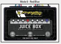
(2008) CBR1000RR 4-2-1 Complete Exhaust Settings: CBR1000RR baseline settings with stock air filter and TBR 4-2-1 Complete system. (G=2.5, Y=5, R=0.5, GB=0.5, YB=5, RB=0.5)
