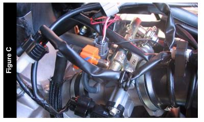
Attach the Juice Box Pro connectors to the stock wiring harness, TPS, and injector as shown in Figure C.
