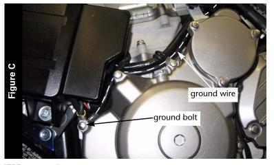
Attach the ground wire from the Juice Box Pro to the common ground on the left hand side of the engine as shown in Figure D.
