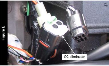
10 Locate the stock O2 sensor connection.
