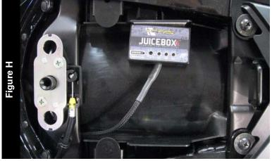
14 Using the supplied velcro, secure the Juice Box Pro in the tail section as shown in Figure H.
