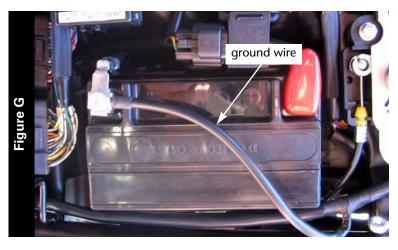
13 Attach the ground wire from the Juice Box Pro to the negative side of the battery as shown in Figure G.
