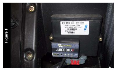
12 Using the supplied velcro, secure the Juice Box Pro to the panel behind the drivers seat above the ECU as shown in Figure F.
