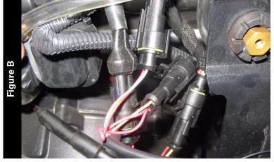
Attach the Juice Box Pro connectors to the injector harness and stock wiring harness as shown in Figure B.
