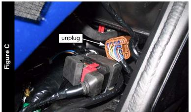
6 Unplug the brown 16-pin main wiring harness connector from the throttle bodies as shown in Figure C.
