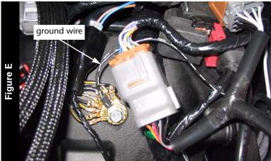
Attach the ground wire from the Juice Box Pro to the stock wiring harness chassis ground as shown in Figure E.
