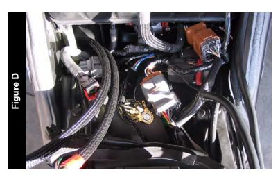
Attach the Juice Box Pro connectors to the throttle body and the stock wiring harness a shown in Figure D.
