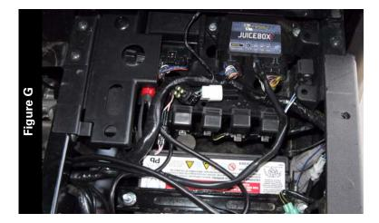
9 Using the supplied velcro, secure the Juice Box Pro to the top of the ECU as shown in Figure G.
