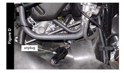
6 Unplug the stock wiring harness from the throttle bodies as shown in Figure D. This is a black 6-pin connector located to the left side of the engine.
