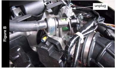
Unplug the grey 2-pin stock wiring harness connector from the injector as shown in Figure B.
