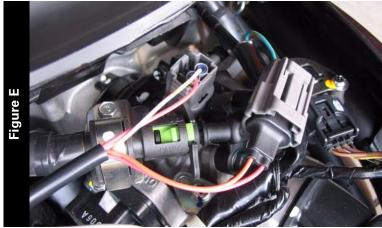
Attach the Juice Box Pro connectors to the injector and stock wiring harness as shown in Figure E.
