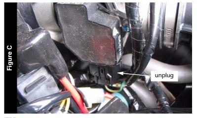
4 Unplug the black 5-pin stock wiring harness from the throttle position sensor (TPS) as shown in Figure C.
