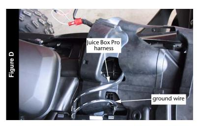
Route the Juice Box Pro harness through the rubber cover as shown in Figure D.
