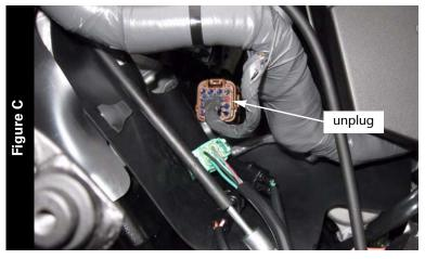
5 Unplug the stock wiring harness from the throttle bodies as shown in Figure C. This is a 16-pin brown connection.
