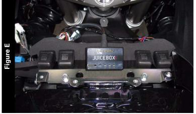
9 Using the supplied velcro, secure the Juice Box Pro to the relay bracket as shown in Figure E.
