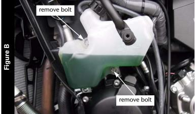
Remove the bolts securing the coolant reserve bottle to the engine as shown in Figure B.
