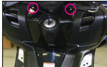
4. Remove foot pad by pulling it upwards to expose bolts, securing right lower cover. (Fig. 3)
