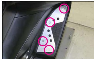
6. Remove mounting hardware from right side lower cover to be able to expose engine and wire harness. (Fig. 5)
