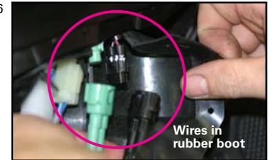
8. Disconnect the green and black two wire connectors one at a time and connect the JUICE BOX™ connectors to these connectors.
