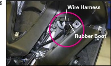
7. Locate rubber boot with 4 wires going inside. (Fig. 6)
