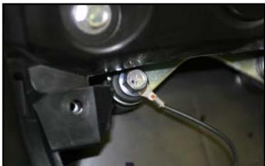
12. Locate and disconnect the BLACK oxygen (lambda) sensor connector. Leave the oxygen sensor connector disconnected. Alternatively, the oxygen sensor may be completely removed from the bike, however an oxygen sensor bung plug (TBR p/n: 005-92-22B) and washer (TBR p/n: 005-92-22W) are required to thread into the OEM or Two Brothers Racing exhaust system where the oxygen sensor was threaded in. (Fig. 11)
