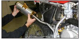
6. Use supplied 8x25mm socket head cap screw for lower frame mount.
