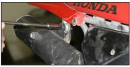
4. Install TBR muffler to TBR slip-on using the supplied 6x14mm socket head cap scews and lock washers provided. Leave loose for now.
