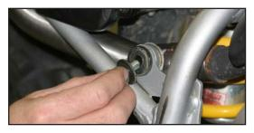
7. Use supplied 8x50mm socket head cap screw for upper muffler mount using the OEM washer and nut. Leave loose for now.
