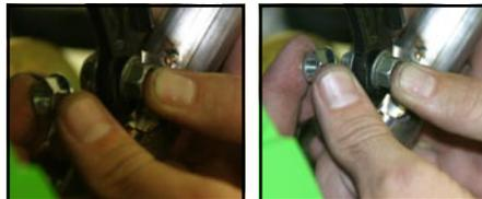
5. Use the supplied 8mm Flange Nut to secure head pipe to mid-pipe bracket using OEM bolt.
