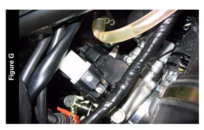
11 Attach the wiring harness from the Juice Box Pro to the stock wiring harness and the TPS as shown in Figure G.
