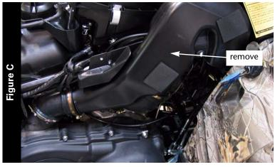
Remove the intake tube for the CVT clutch on the right hand side of the quad as shown in Figure C.
