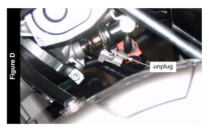
Unplug the stock wiring harness from the injector as shown in Figure D. Figure D was taken from the left hand side of the quad.
