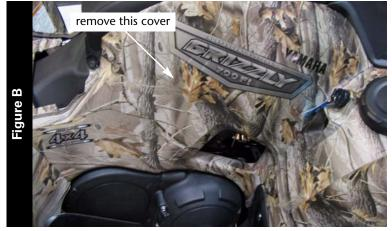
Remove the right hand side cover as shown in Figure B. Remove the same cover on the left side.
