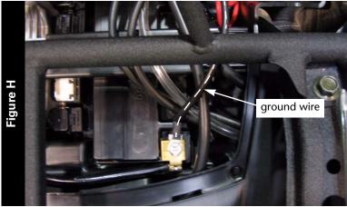
12 Attach the ground wire from the Juice Box Pro to negative side of the battery as shown in Figure H.
