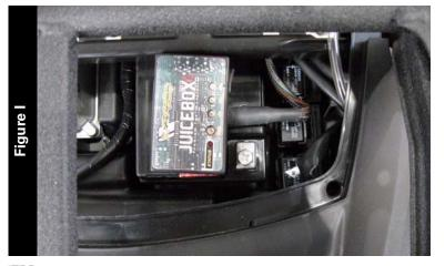
13 Using the supplied velcro, secure the Juice Box Pro to the battery as shown in Figure I.
