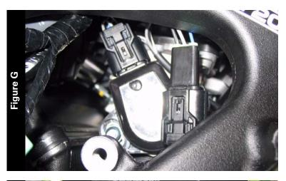
12 Attach the black connectors from the Juice Box Pro to the stock TPS and wiring harness as shown in Figure G.
