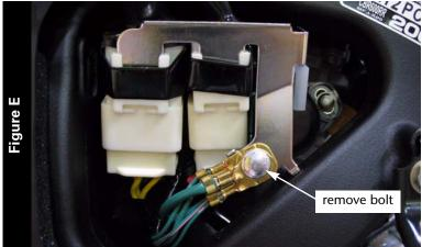
10 Remove the bolt holding the ground wires and bracket for the alternator connectors to the frame on the left hand side of the bike.
