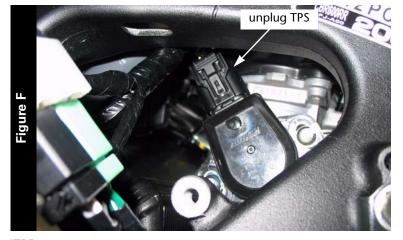
11 Unplug the stock wiring harness from the throttle position sensor (TPS) as shown in Figure F.
