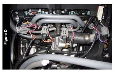
Attach the Juice Box Pro connectors to the stock injectors and stock wiring harness as shown in Figure D.
