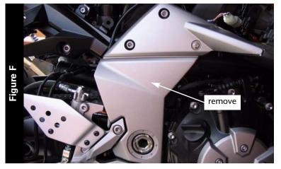
11 Remove the frame cover on the right hand side as shown in Figure F.
