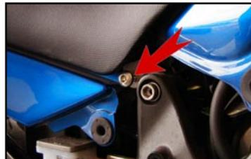
5. Remove the front (2) tank bolts (Fig 4).
