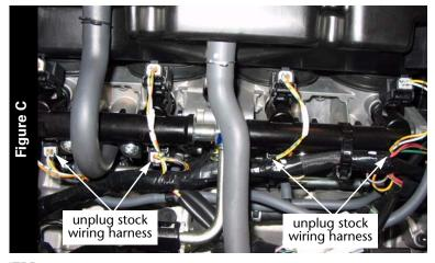
7 Unplug the stock wiring harness from each of the lower injectors as shown in Figure C.
