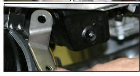
Use small amount of hightemp silicone on the inside of collector left and collector right and install onto headers. They are stamped CL and CR.
