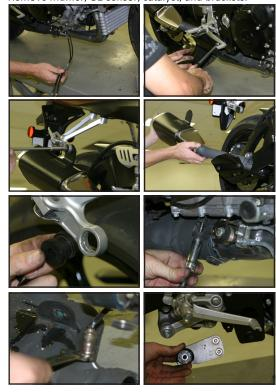
Remove OEM headers, this may require to move oil cooler and radiator for easier access.
