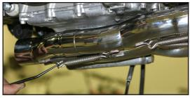
12. Attach 2 part X-Ring to muffler by loosely attaching one side and slipping the mid-pipe under retaining ring then install the second part and leave loose for now.
