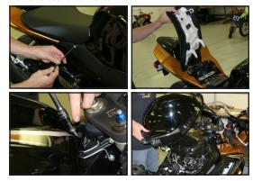
Remove servo and servo bracket. Replace with supplied bracket and servo stop (be sure to hold servo wheel when removing so damage to internals does not occur).
