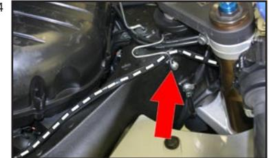
8. Disconnect the LOWER injector connectors from the LOWER injectors. Connect the JUICE BOX™ female and male connectors to the injectors and the injector connectors that were just disconnected. Do NOT connect the JUICE BOX™ to the upper injector connectors. (Fig 5)
