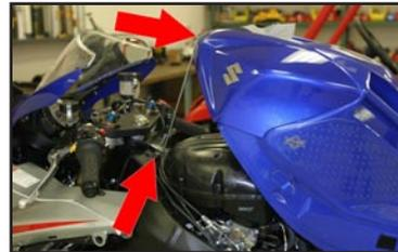
6. Attach the adhesive backed hook and loop material to the back of the JUICE BOX™ and the front sub-frame below the instrument cluster. (Fig 3)
