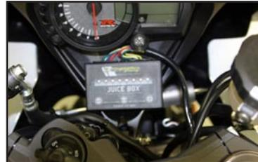
7. Route the JUICE BOX™ harness between the steering stem and the right fork tube. Remove the bolt securing the harness guide bracket and route the JUICE BOX™ harness through the harness guide bracket and down the right side of the air box to the lower fuel injection rail. (Fig 4)
