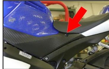
3. Remove the front seat. Remove the tank side panels by holding the rear of the panel and gently pulling out and back.
