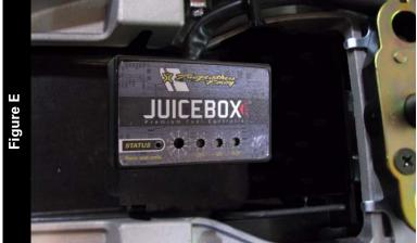
12 Using the supplied velcro, secure the Juice Box Pro in the tail section as shown in Figure E.
