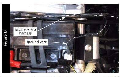
11 Attach the ground wire from the Juice Box Pro to the negative side of the battery as shown in Figure D.
