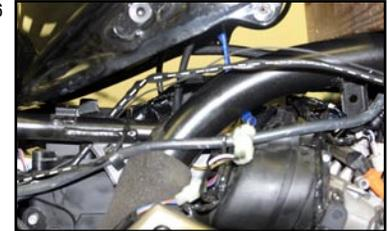
8. Attach the adhesive backed hook and loop material to the back of the JUICE BOX™ and side of the storage compartment under the front seat. (Fig 7)
