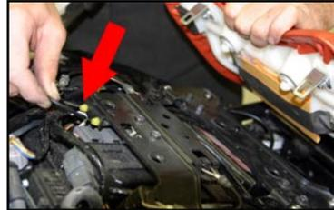
4. Remove the bolt that secures the small right side tank cover and gently pop the cover off. Repeat for left side. (Fig 3)
