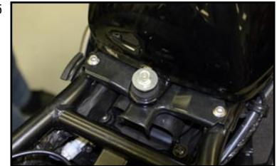
7. Route the JUICE BOX™ harness from the storage compartment under the front seat to the fuel injector connectors. (Fig 6)
