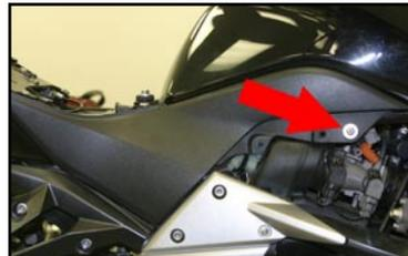
6. Remove rear tank mount bolt and gently slide tank toward the rear of the bike. Prop the tank up exposing the fuel injector connectors. (Fig 5)
