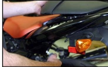
3. Remove the front seat by pulling the loop and lifting the front seat. (Fig 2)
