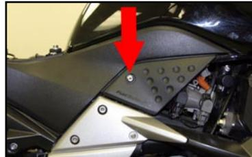
5. Remove the bolt that secures the large right side tank cover and gently pop the cover off. Repeat for left side. (Fig 4)
