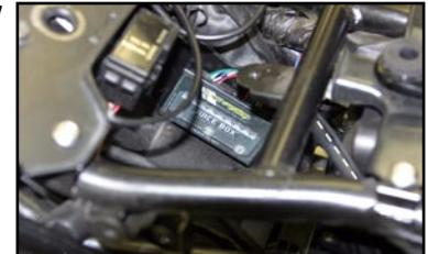
9. Disconnect the injector connectors from the injectors. Connect the JUICE BOX™ female and male connectors to the injectors and the injector connectors that were just disconnected. (Fig 8)
