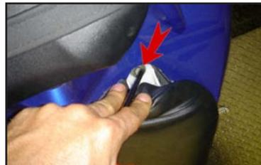
4. Remove bolt at front and center of fuel tank (fig 3)
