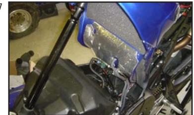
8. Locate four grey injector connectors at the rear of the air box, under the fuel rail. (fig 8)
