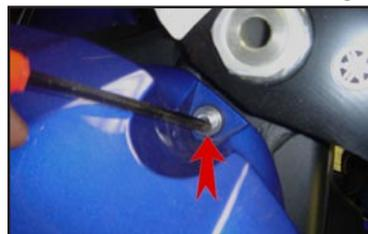
5. Remove both Phillips screws at the right rear and left rear of fuel tank lower trim panels. The panel is an interlock type, slide front to back to release. (fig 4 & 5)
