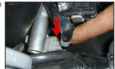
9. Remove grey injector connectors one at a time and connect JUICE BOX™ grey connectors to injectors and connect JUICE BOX™ black connectors to stock grey connectors. Repeat this step for all four injectors. (fig 9)
