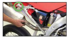
Apply threadlock to the 4 (four) 6mm x 16mm bolts and loosely attach the X-Lite™ ring to muffler inlet.
