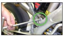
9. Securely tighten the 4 (four) 6mm x 14mm hex head bolts of the V.A.L.E. assembly.
