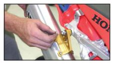
8. Using the supplied 8x16mm flange bolt, secure muffler assembly mid-pipe bolt. Tighten securely.
