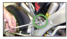
4. Remove upper muffler mounting bolt and muffler assembly.
