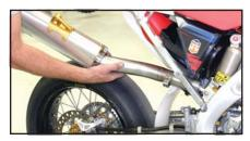
7. Attach muffler mounting bracket to mounting tab on subframe using supplied 8x25mm bolt. Leave loose for now.
